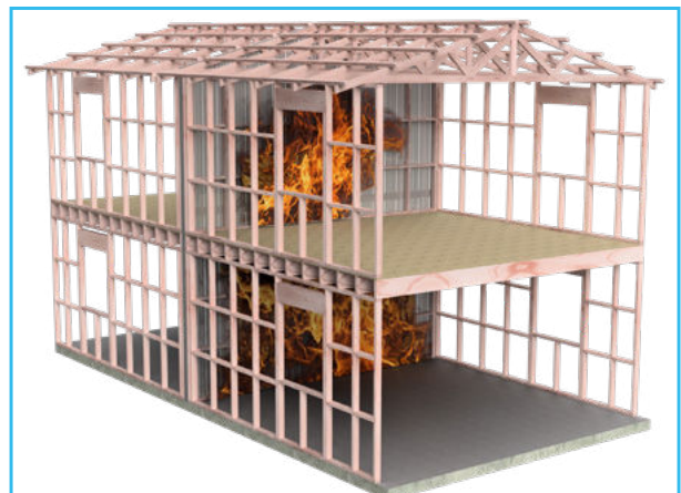
DURING FIRE - KOROK® aluminium brackets on the fire side melt.
