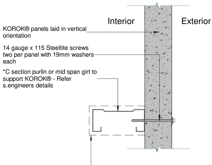
\*In order to satisfy the requirements of the New Zealand Building Code (clause C6) relating to "structural stability during fire" designers must ensure that KOROK® elements are supported by primary elements that have at least the same fire rating as the KOROK® system that is used.
